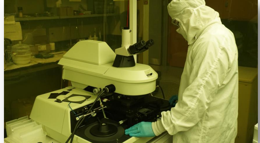
UV exposure of gold layer to form patterned electrode
