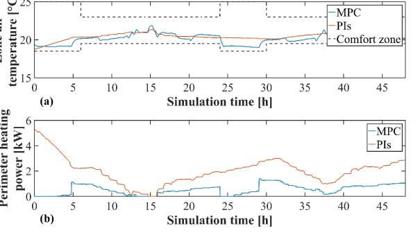
(a) Zone 10 air temperature and (b) perimeter heating power consumption during the simulated time in winter.
