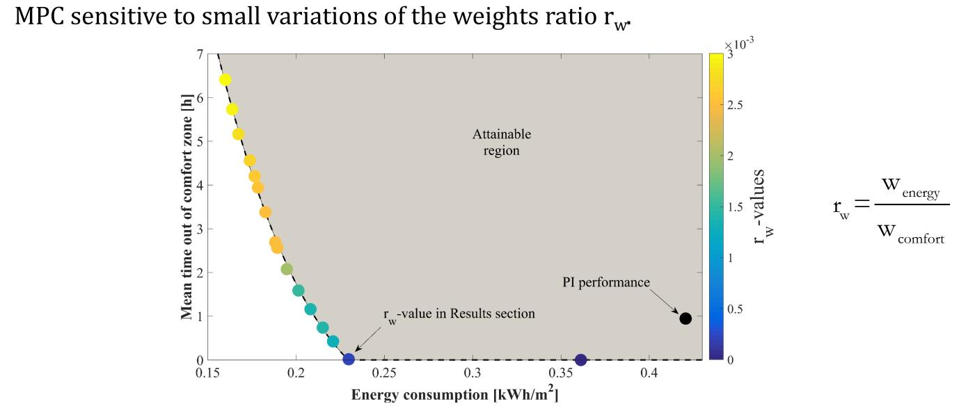
Optimized energy consumption and thermal comfort as a function of the relative importance given to each objective.
