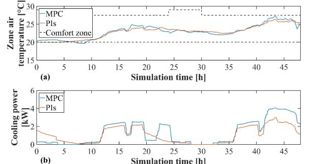
(a) Zone 10 air temperature and (b) rooftop unit cooling power consumption during the simulated time in summer.
