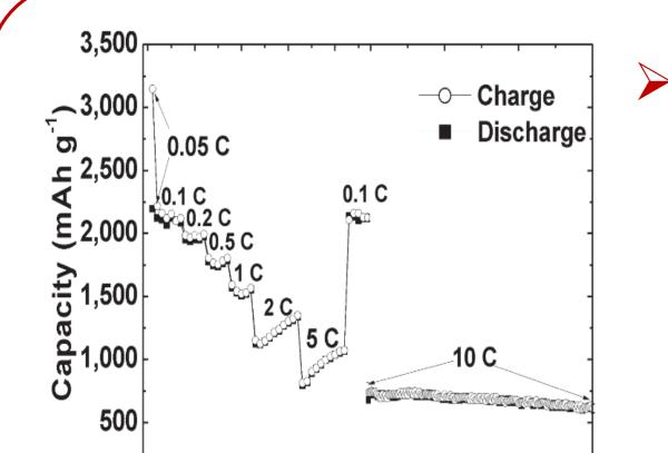
The nanostructured Silicon/ Reduced Graphene Oxide (Si/RGO) electrode remains high charge/discharge capacities even at high C-rate (87% at 10 C).
